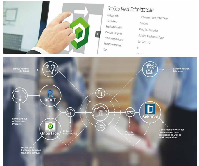
Fig. 3. The interface can be used to import specific building components into BIM models
